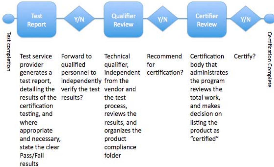
Figure 16 – Conformance and Interoperability Certification Testing – Part 2
